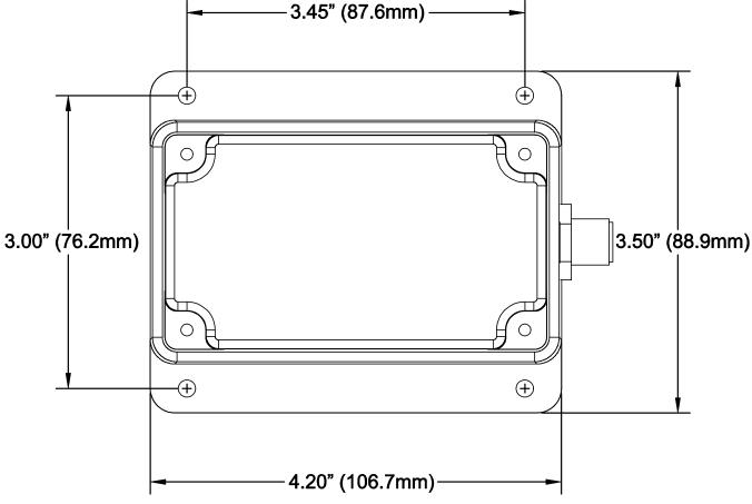
Figure 6 – Mounting Surface Template
